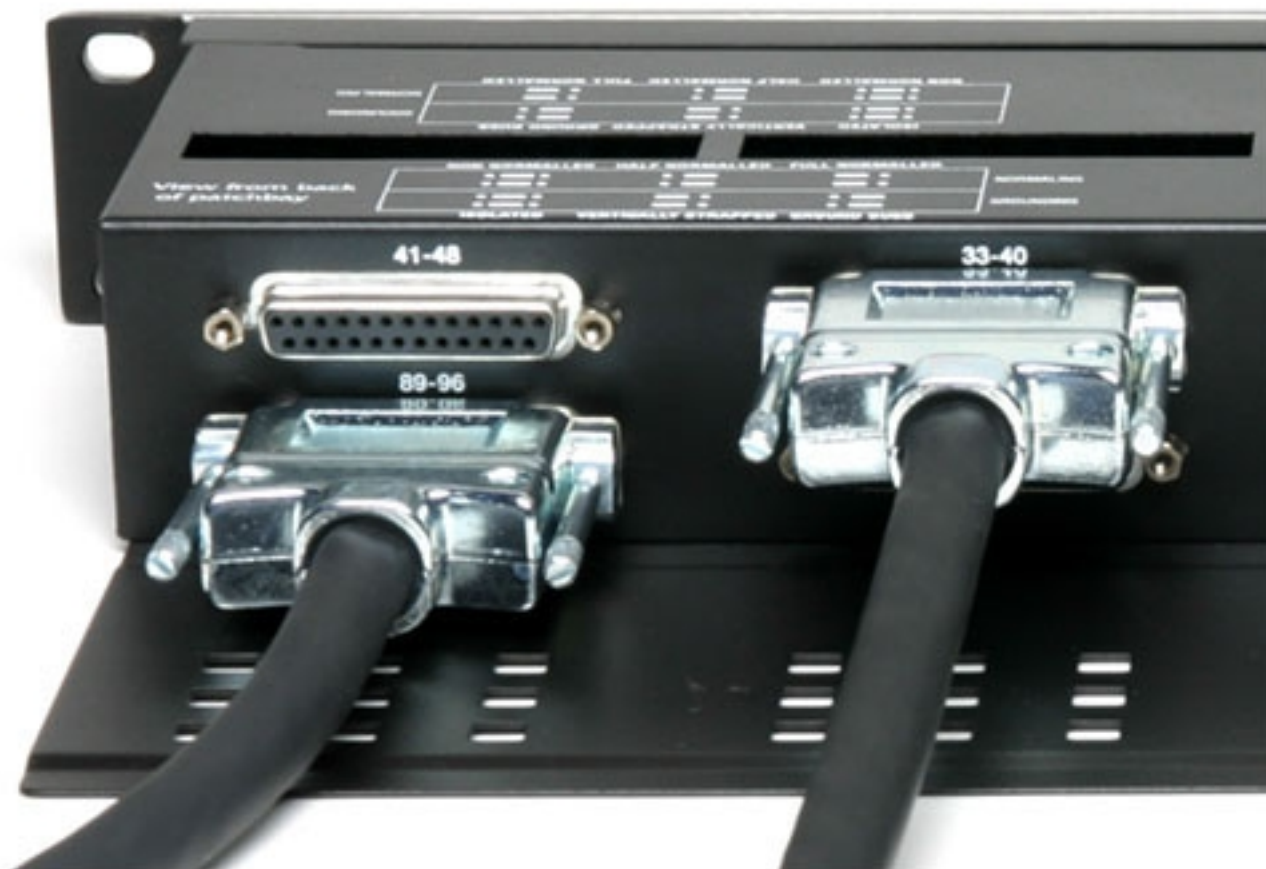
Illustration 7: Here's the back of the Redco TT/DB25.
