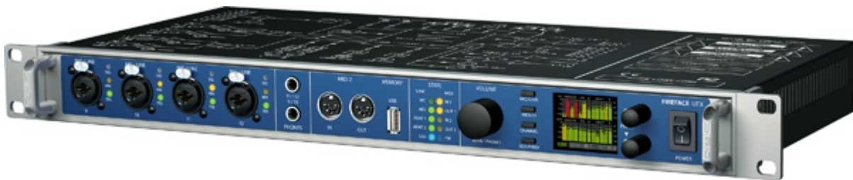
Illustration 2: In this build, we are going to replace my Toft ATB32 with this RME UFX's internal Totalmix FX mixer.
